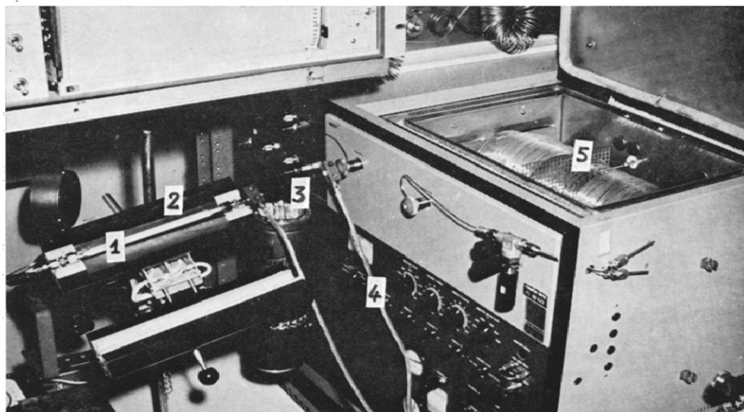
Fig. 3. Actual configuration of elution system. 1 = Tenax column; 2 = oven; 3 = U-tube condenser; 4 = flash heater cables; 5 = dual-column gas chromatograph.
